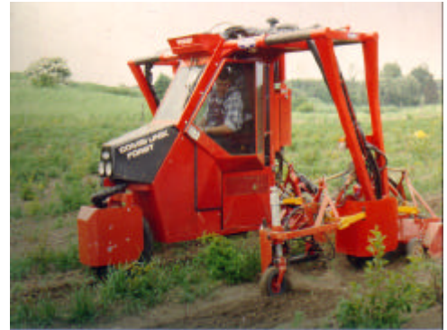
Fig. 1. A self-propelled row weeder for Christmas trees (courtesy: A. Bergstedt)
